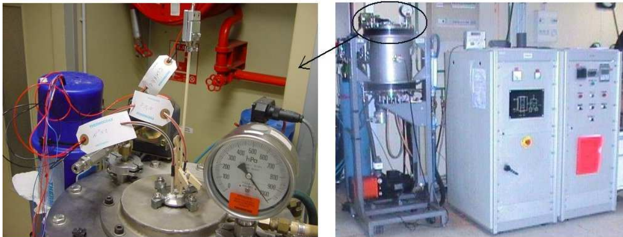
Figure 4: detailed and general views of the 2000°C THERMOCOAX furnace used for high-temperature studies
